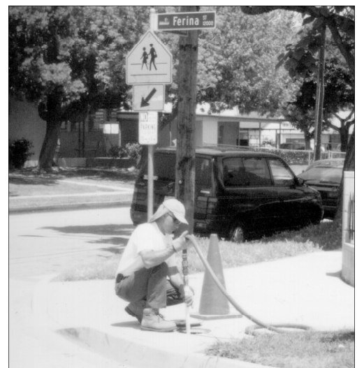
Semi-Annual Monitoring. A contractor prepares a monitoring well for water purging prior to the April groundwater sampling event.
